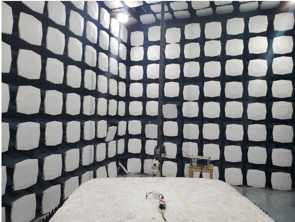
Picture 1 Radiated Emission Test Setup
