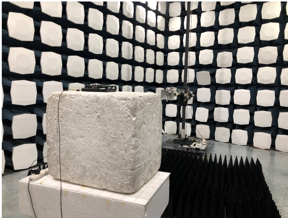
Picture 1 Radiated Emission Test Setup
