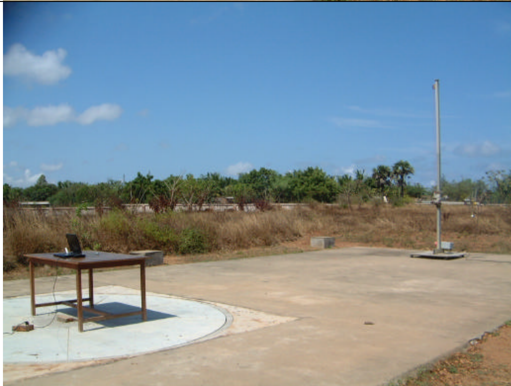
Radiated emission test setup vertical polarization
