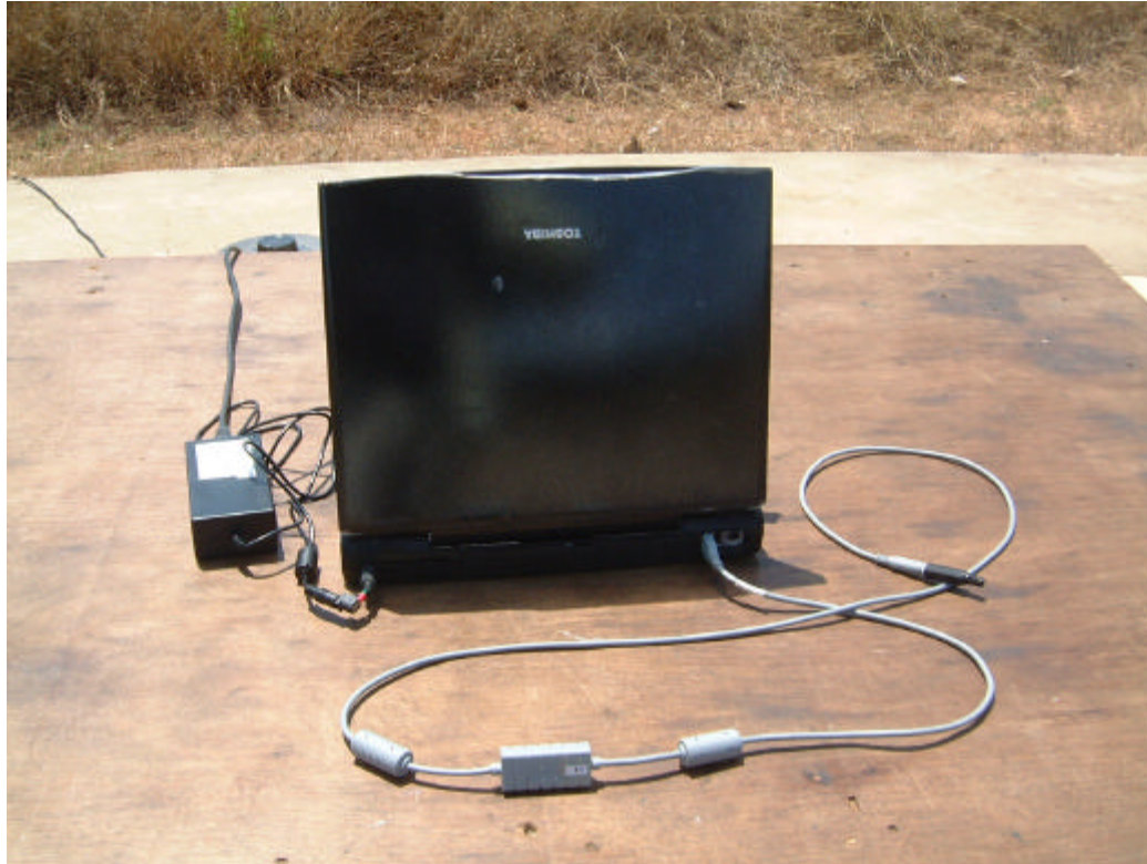
Radiated emission test setup at Open area test site. (Photograph shows maximum emission position of the cable)
