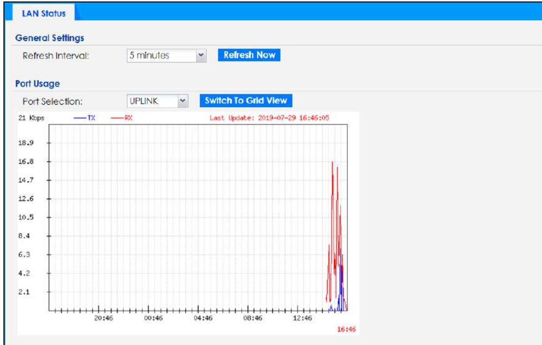
Figure 38 Monitor > Network Status > Switch to Graphic View
