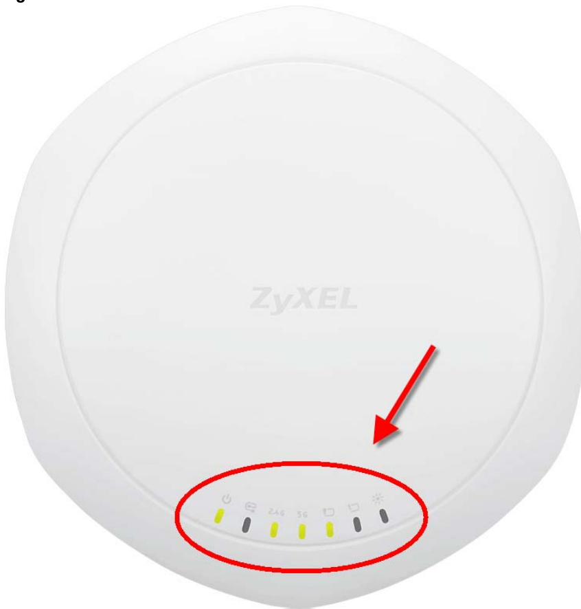
Figure 23 NWA1123-AC PRO LEDs
