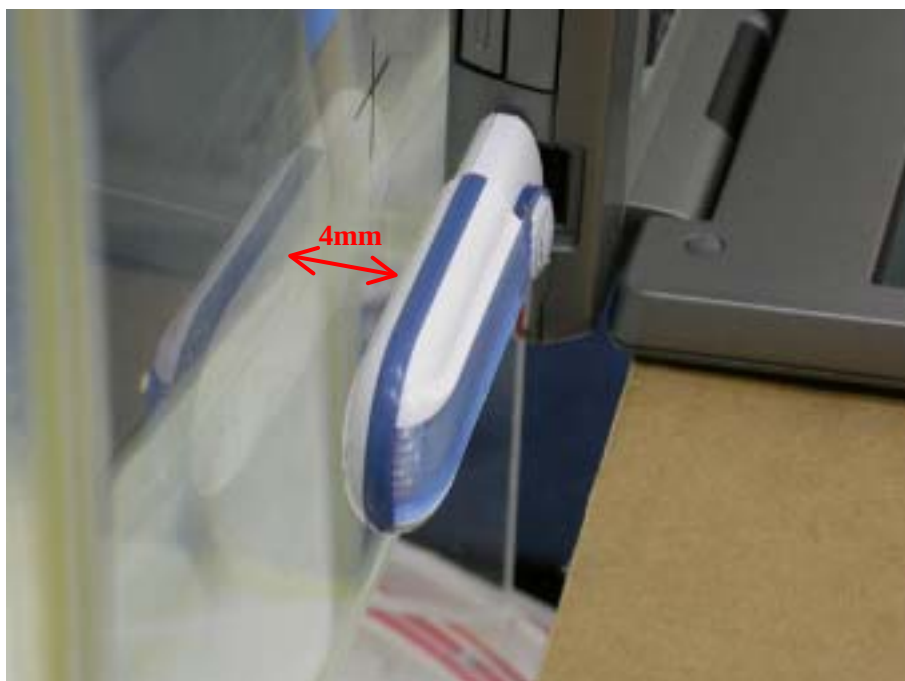
Figure 3: Bottom side of Laptop facing phantom touching - Zoom In
