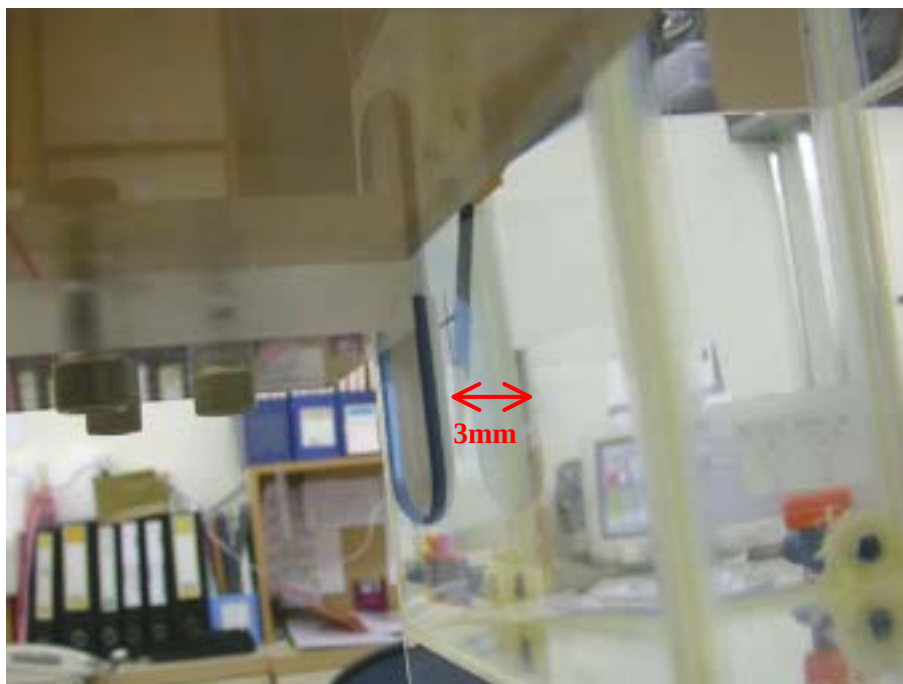
Figure 15: Bottom side of Laptop facing phantom touching-Zoom In
