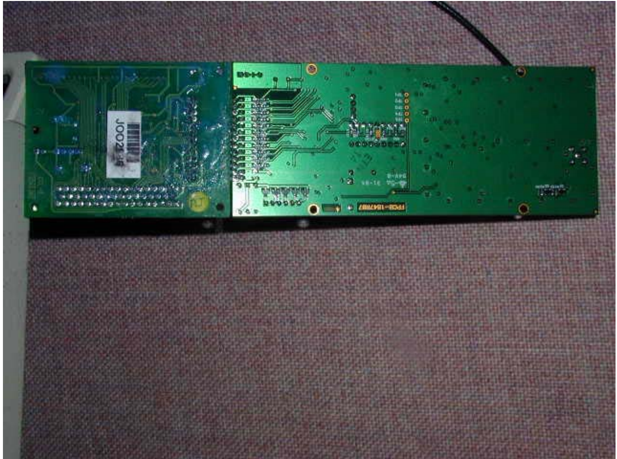
BACK OF RF BOARD
