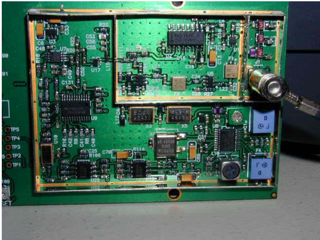
RF BOARD RIGHT PART WITHOUT CAN
