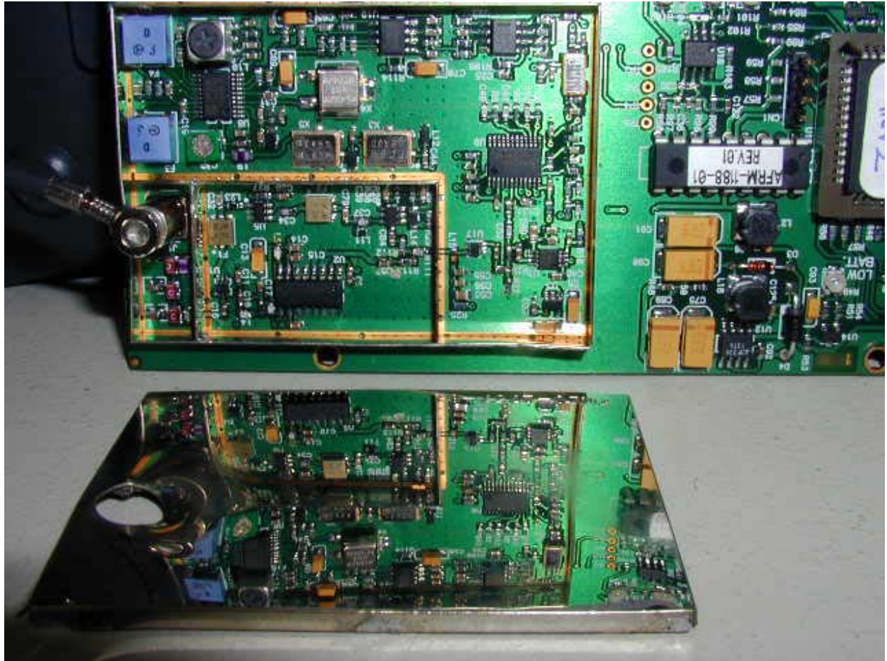
RF BOARD RIGHT PART WITH CAN
