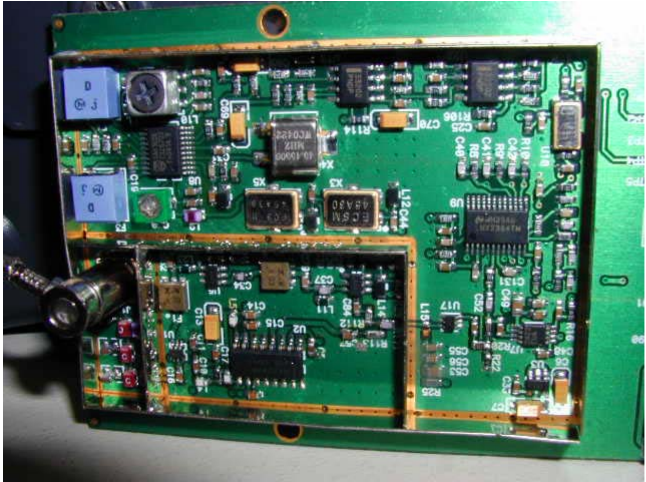
RF BOARD RIGHT PART WITHOUT CAN
