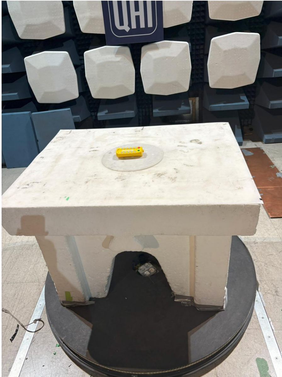
Radiated Emissions – 30MHz to 1GHz – Horizontal Orientation
