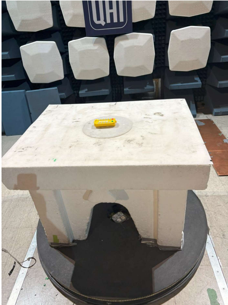
Radiated Emissions – 30MHz to 1GHz – Horizontal Orientation
