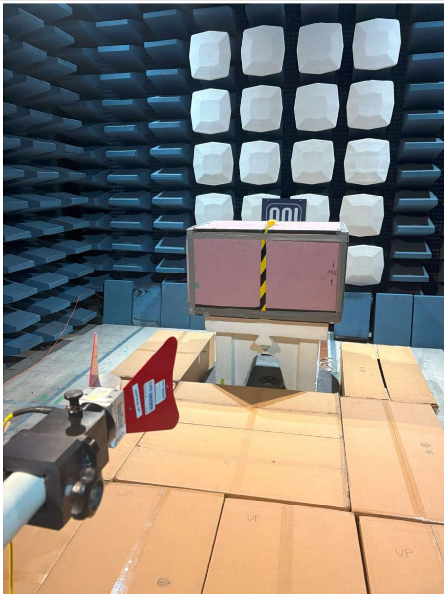
Radiated Emissions – 1GHz to 18GHz – Horizontal Orientation
