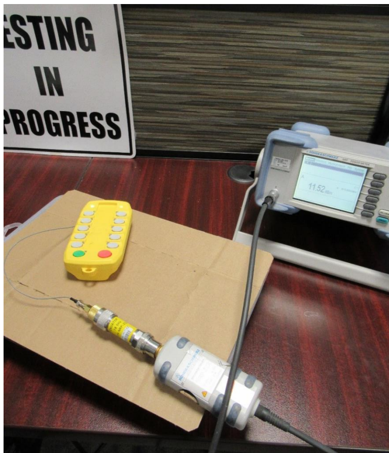
Figure 4: Max Peak Conducted Output Power Measurements
