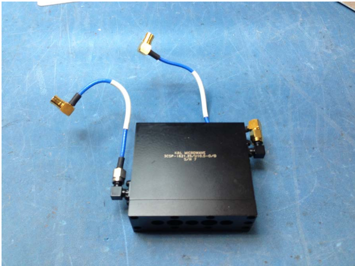
Figure 6: Cavity Filter Top
