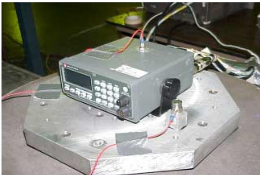
Figure 3-4. Test setup for vertical-axis sinusoidal vibration.
