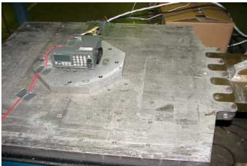
Figure 2-4. Test setup for lateral-axis sinusoidal vibration.
