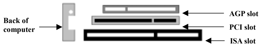
AGP vs. PCI vs. ISA expansion slots
