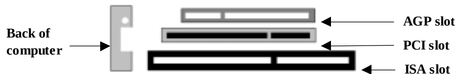
AGP vs. PCI vs. ISA expansion slots
