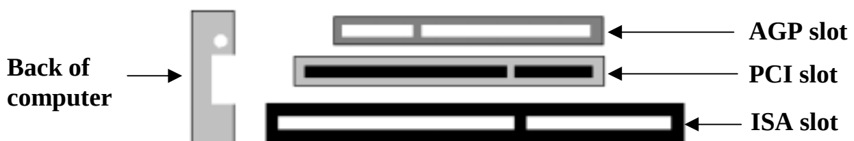
AGP vs. PCI vs. ISA expansion slots
