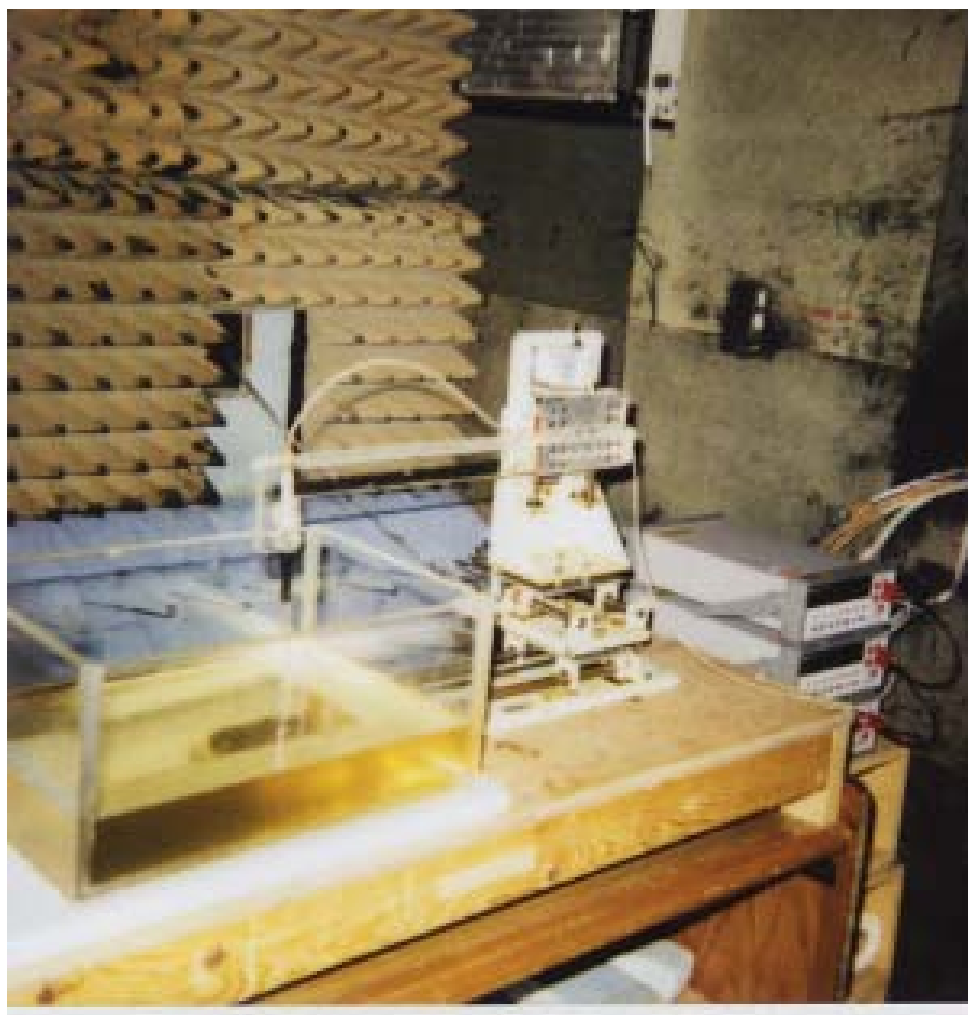
Fig. 5. Photograph of the three-dimensional stepper-motor-controlled SAR measurement system using a planar phantom (see Figs. 3 and 4 for a detailed examination of the placement of Tablet PC relative to this phantom).
