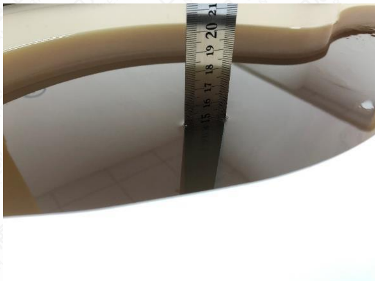
Figure 9.2-1 Liquid depth in the Flat Phantom for SAR measurements \leq 3 \text{ GHz}
