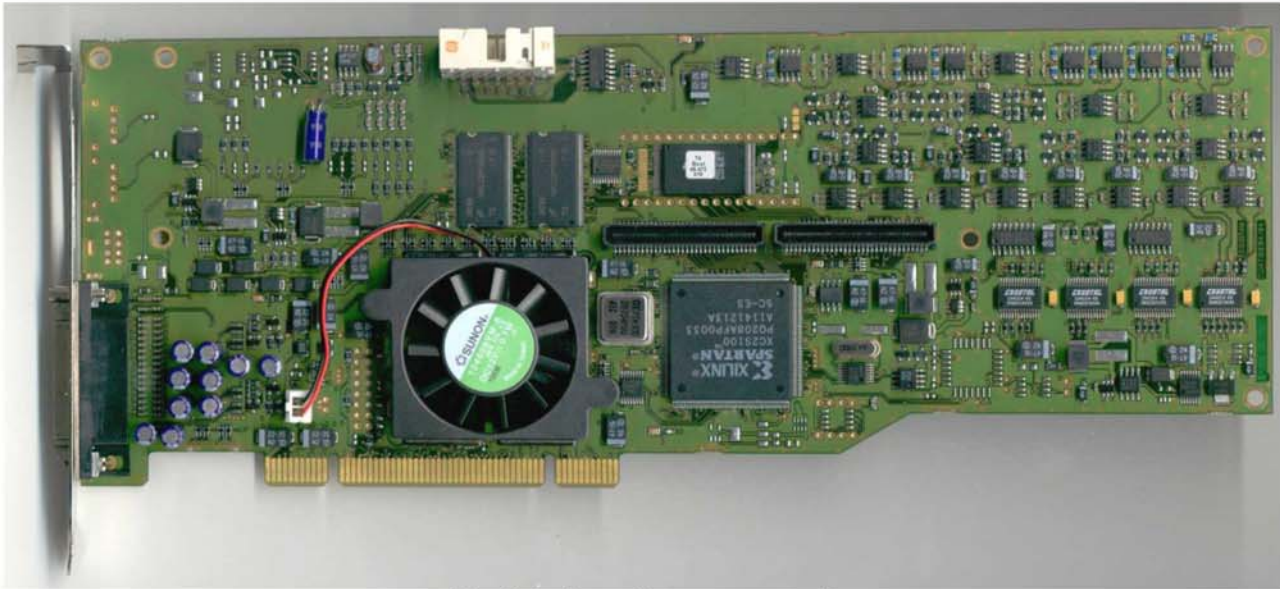
miXart8 (main card), components side.
