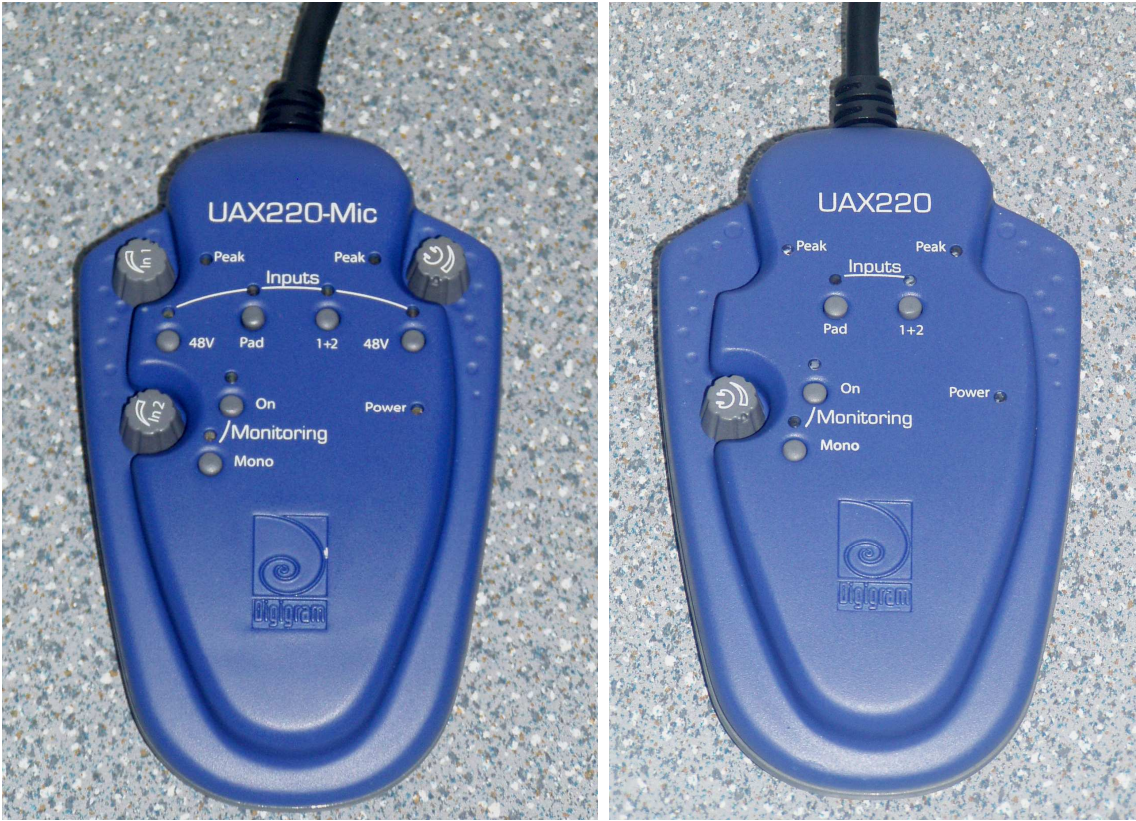
Detail view, upper face (UAX220-MIC & UAX220v2)
