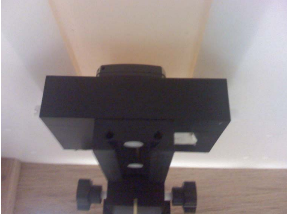
Figure 8 - Transceiver against body, 25 mm from Phantom position
