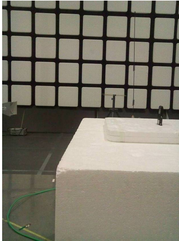
23156-1, IHDP56KB1 setup in semi-anechoic chamber – right view (18 GHz – 26.5 GHz)
