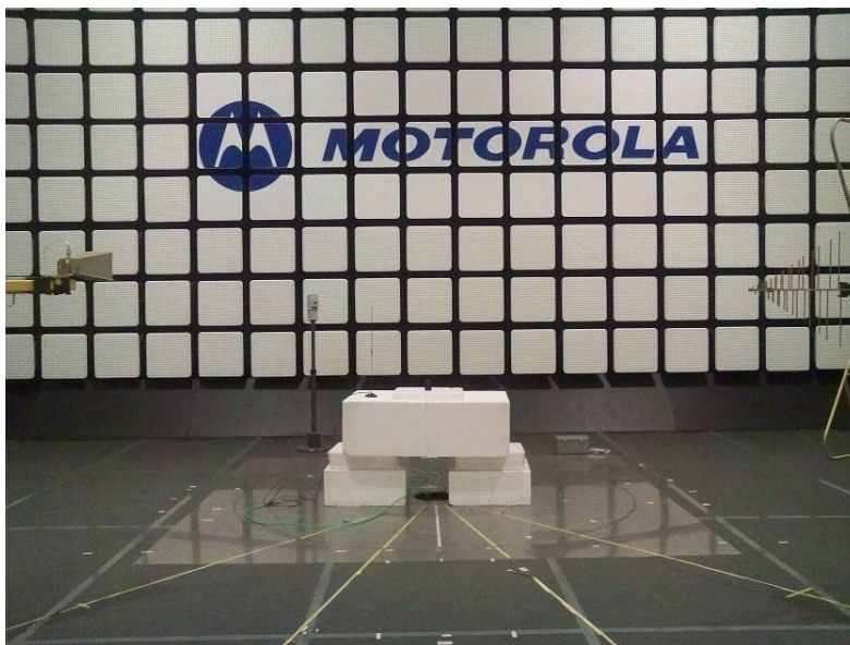
23156-1, IHDP56KB1 setup in semi-anechoic chamber – front view (30 MHz – 18 GHz)
