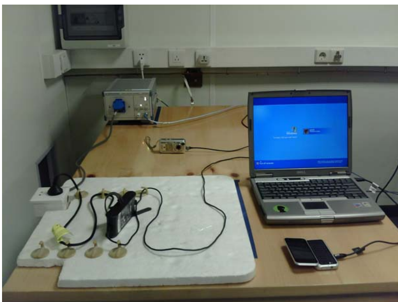
AC Line Conducted Emissions – Computer Peripheral
