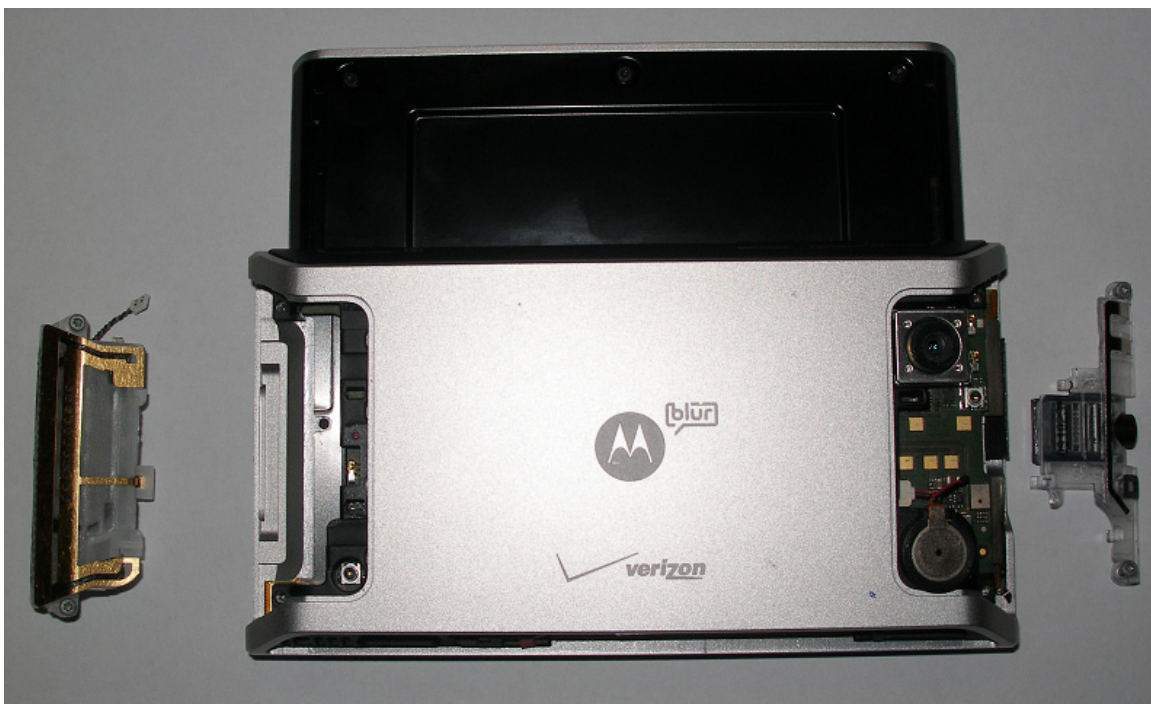
Rear View Antenna carriers off
