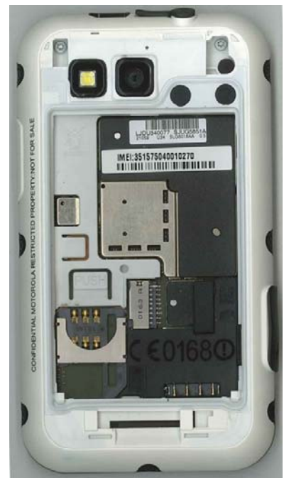
Back of Phone Battery cover removed.
