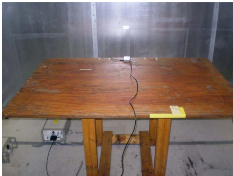
BT AC Line Conducted Emissions
