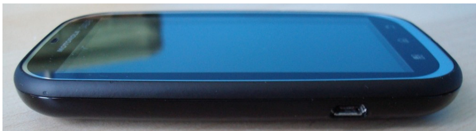
Left Side of the Phone (Micro USB Connector)
