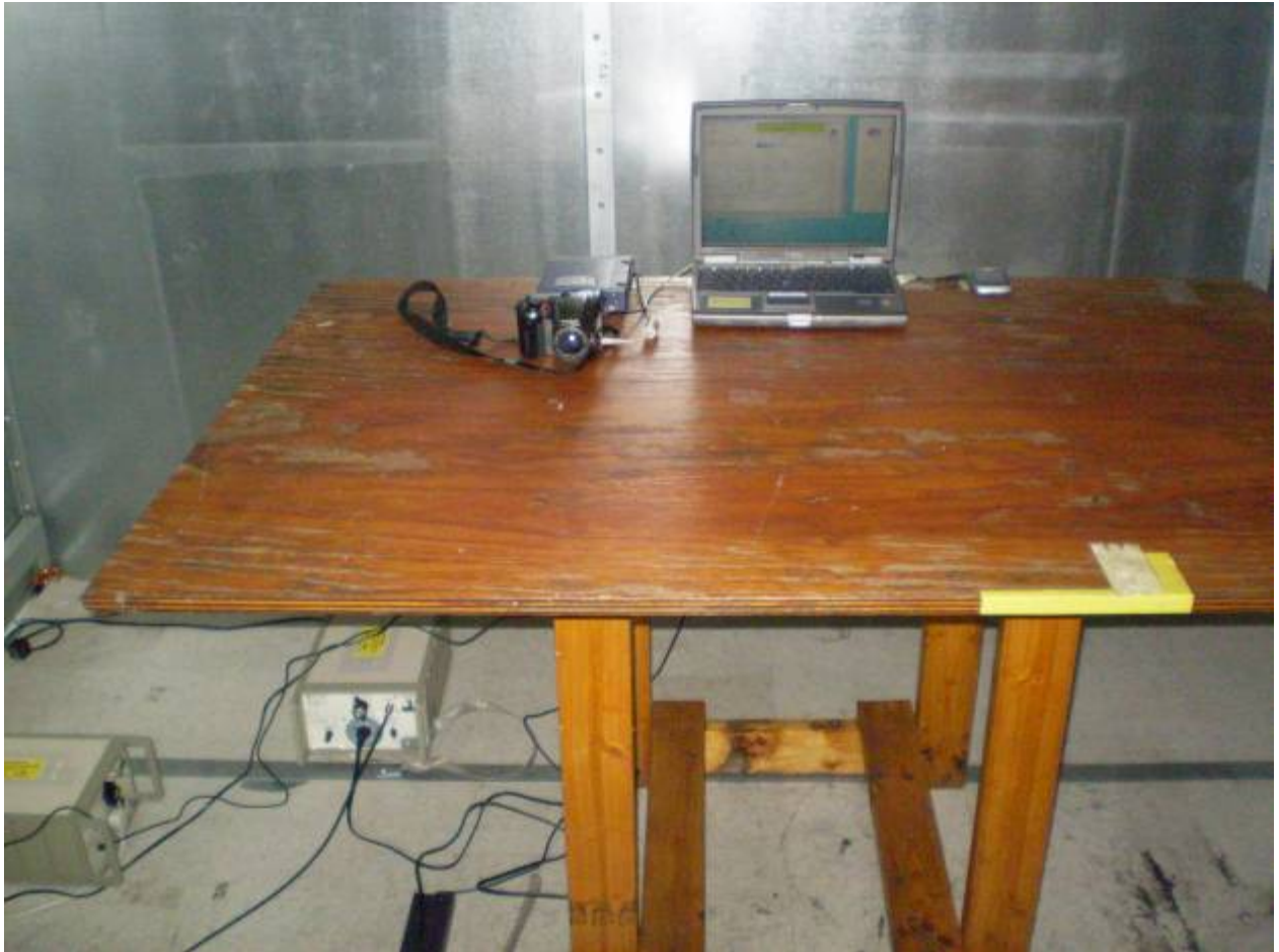
AC Line Conducted Emissions
