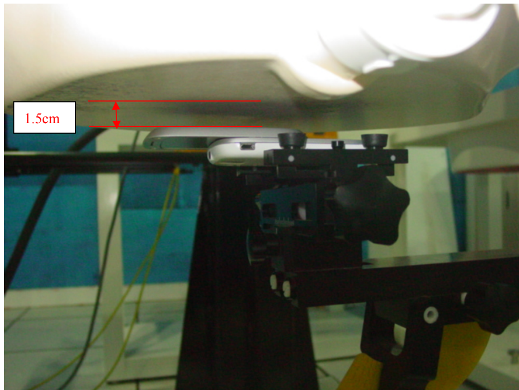
Picture B16: Body-worn Position (towards phantom, the distance from handset to the bottom of the Phantom is 1.5cm) – Slide up
