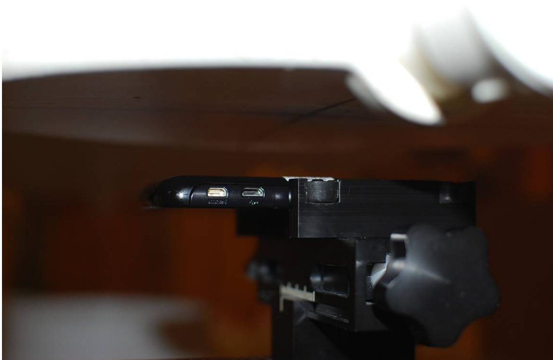
Figure 18-2 SAR Test Setup Back 2.5 cm
