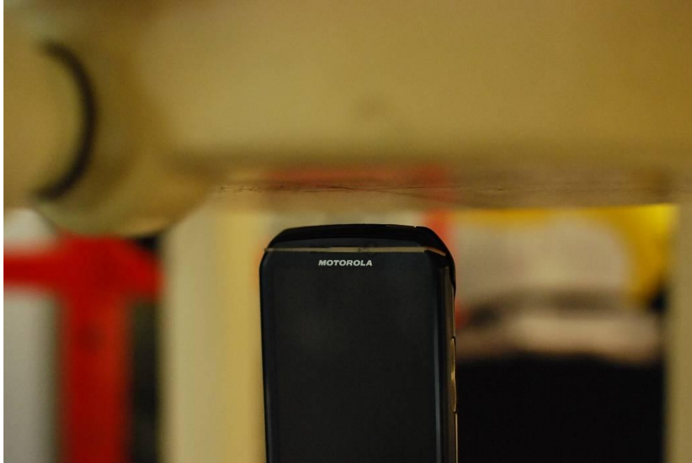
Figure 24-7 SAR Test Setup Photo – Top at 1.0 cm
