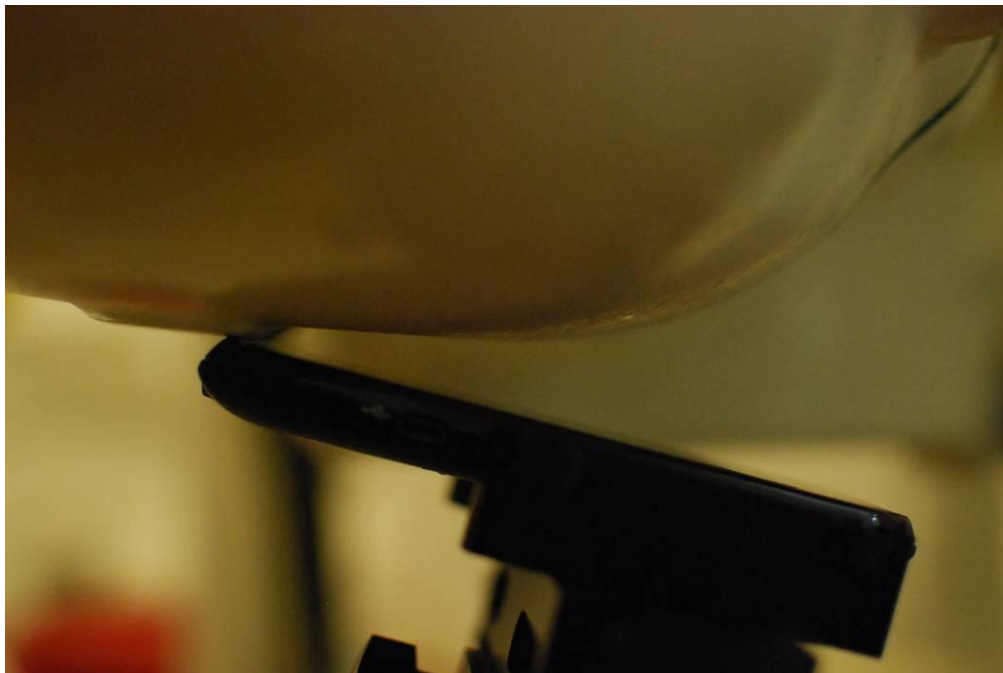
Figure 24-2 SAR Test Setup Photo – Right Tilt
