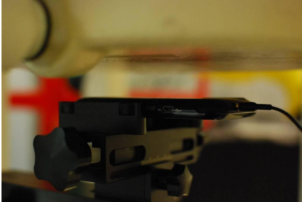
Figure 24-11 SAR Test Setup Photo – Body-Worn at 2.5 cm
