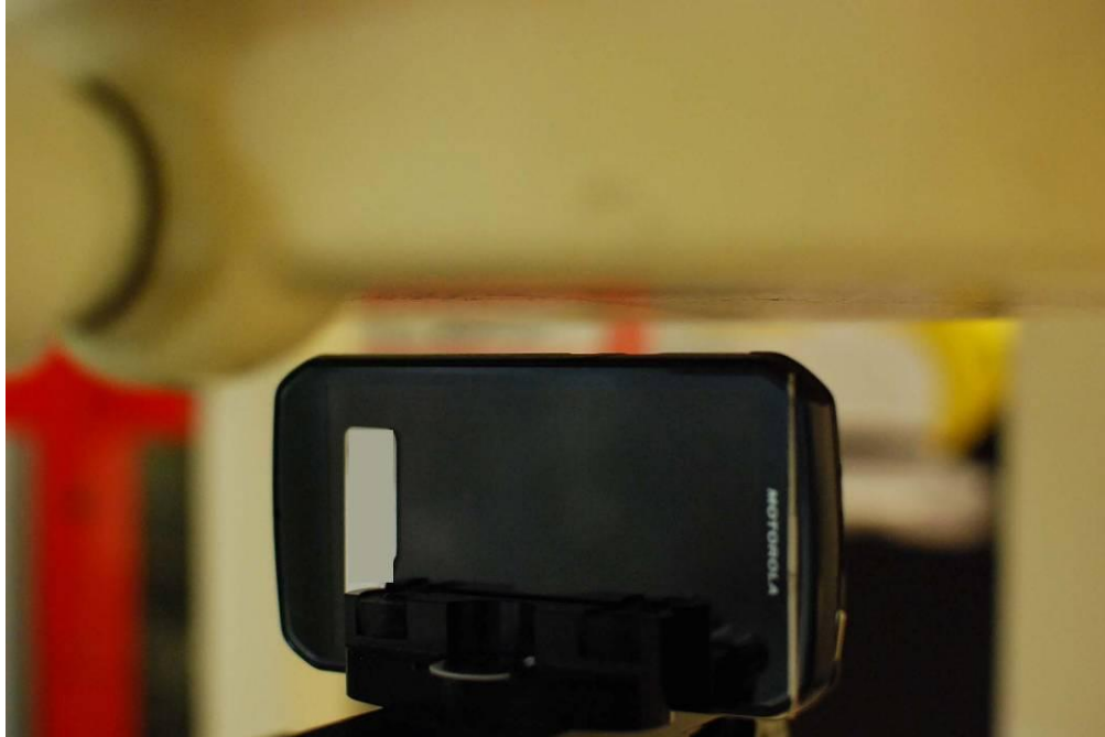
Figure 24-9 SAR Test Setup Photo – Left at 1.0 cm
