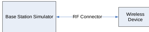
Figure 11-1 Power Measurement Setup
