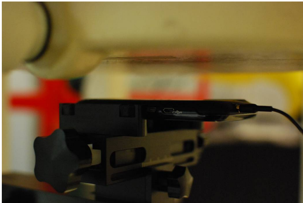
Figure 22-10 SAR Test Setup Photo – Body-Worn at 2.5 cm
