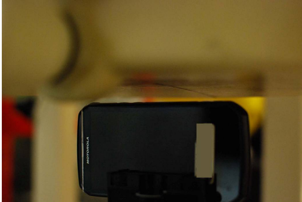
Figure 22-9 SAR Test Setup Photo – Right at 1.0 cm
