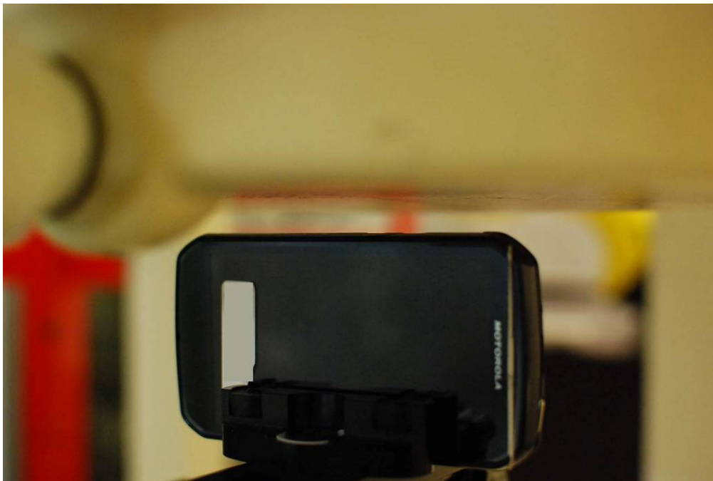
Figure 22-8 SAR Test Setup Photo – Left at 1.0 cm
