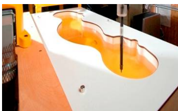
Figure 6-2 SAM Phantom with Simulating Tissue
