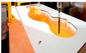
Figure 6-2 SAM Phantom with Simulating Tissue
