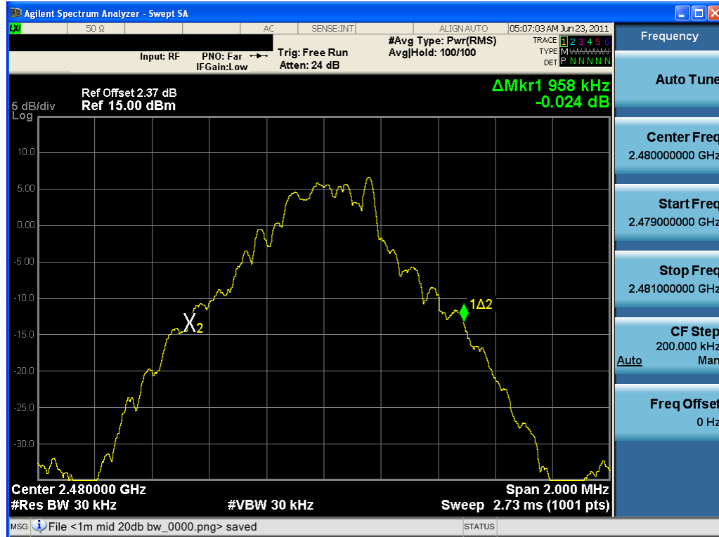
Plot 6-3. 20dB Bandwidth Plot (Bluetooth, 1Mbps – Ch. 78)
