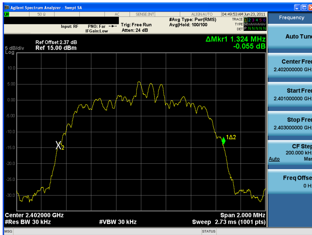
Plot 6-4. 20dB Bandwidth Plot (Bluetooth, 2Mbps – Ch. 0)
