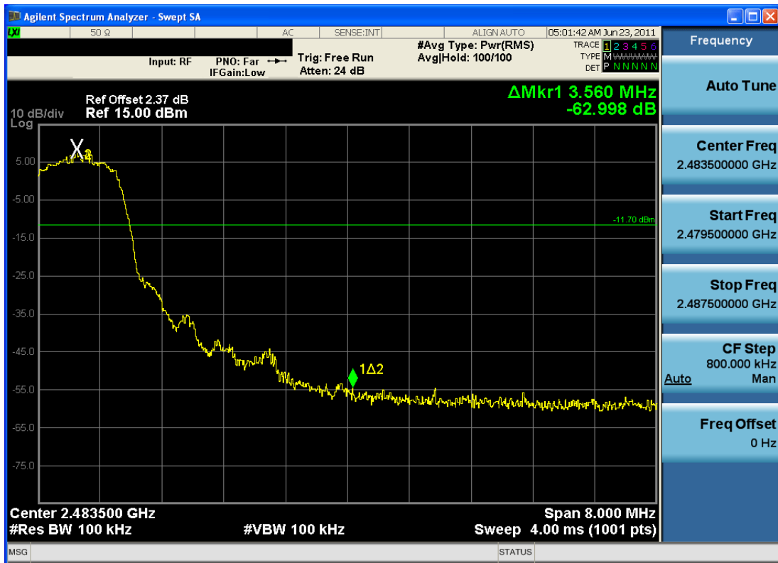
Plot 6-13. Band Edge Plot (Bluetooth, 2Mbps – Ch. 78)
