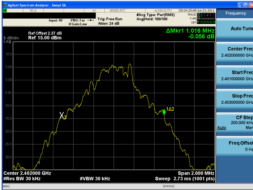
Plot 6-1. 20dB Bandwidth Plot (Bluetooth, 1Mbps – Ch. 0)
