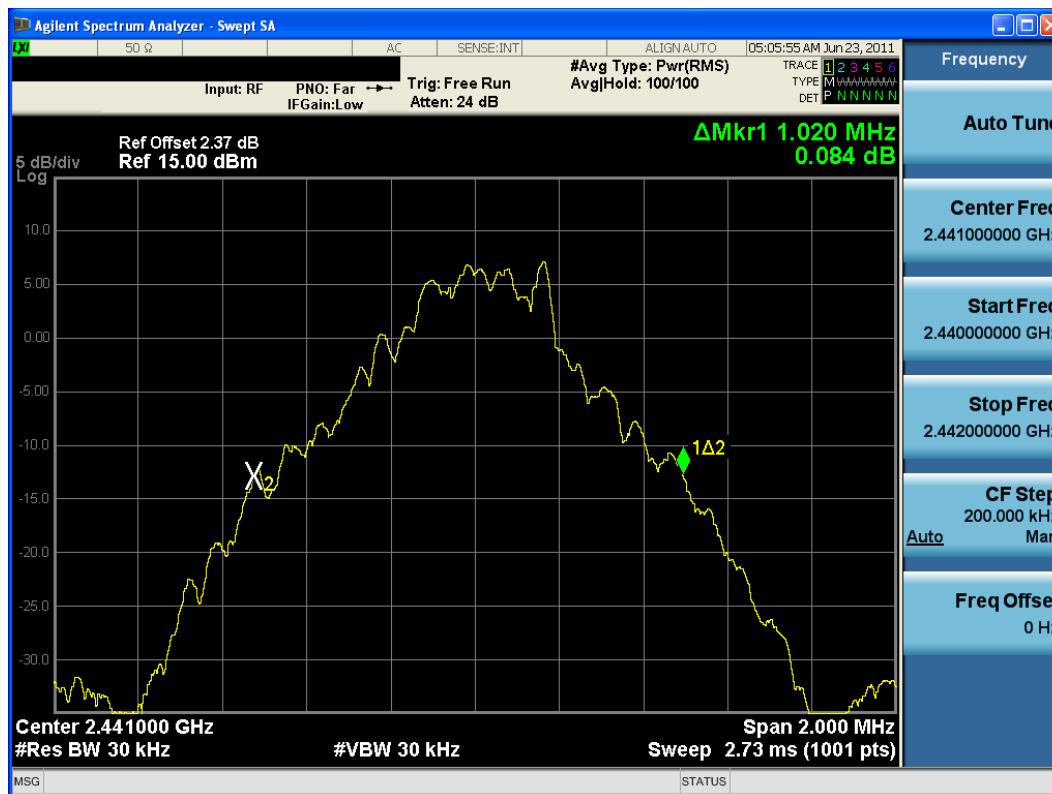
Plot 6-2. 20dB Bandwidth Plot (Bluetooth, 1Mbps – Ch. 39)
