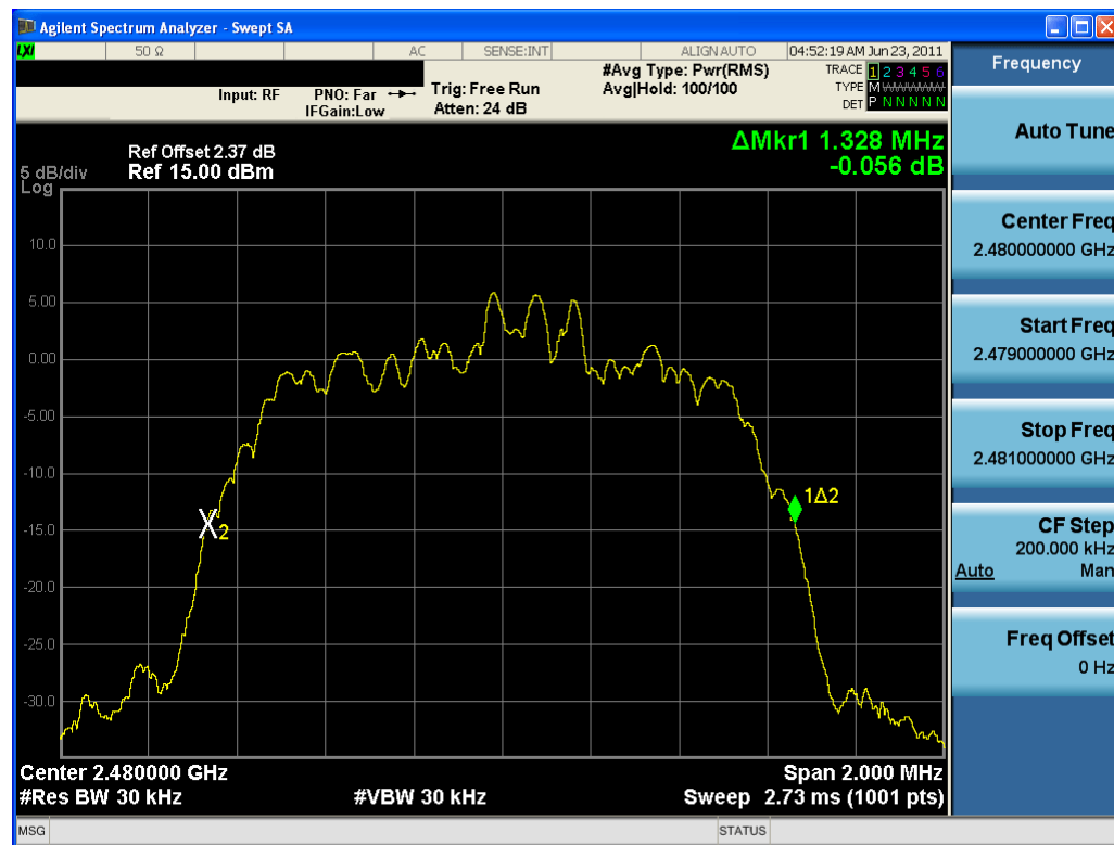
Plot 6-6. 20dB Bandwidth Plot (Bluetooth, 2Mbps – Ch. 78)
