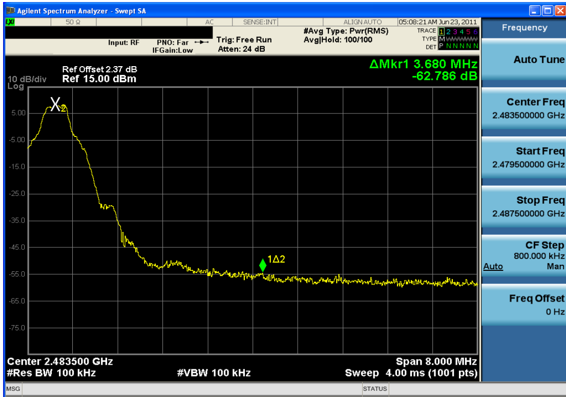
Plot 6-11. Band Edge Plot (Bluetooth, 1Mbps – Ch. 78)
