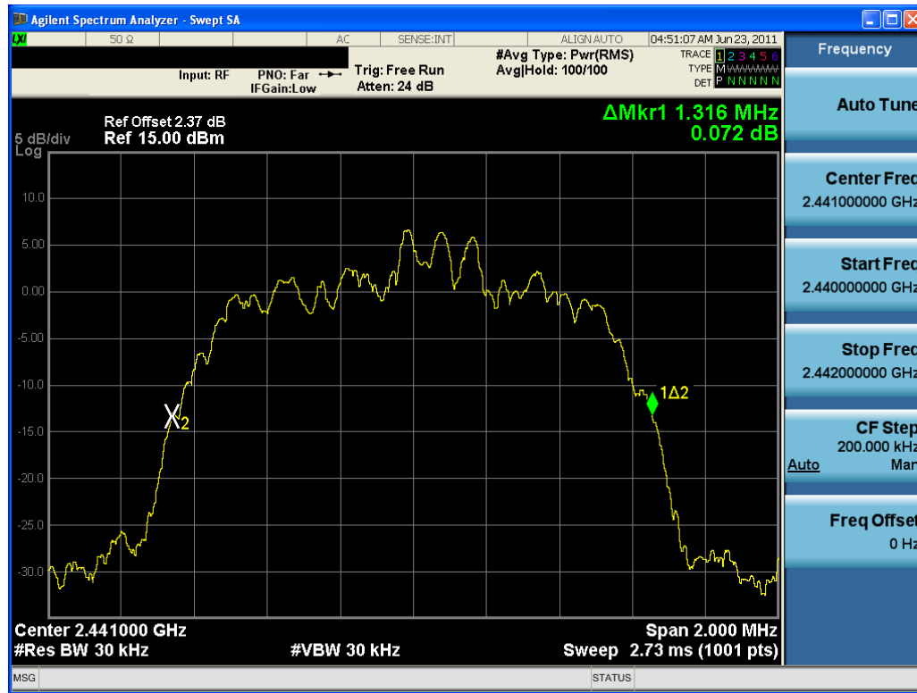
Plot 6-5. 20dB Bandwidth Plot (Bluetooth, 2Mbps – Ch. 39)
