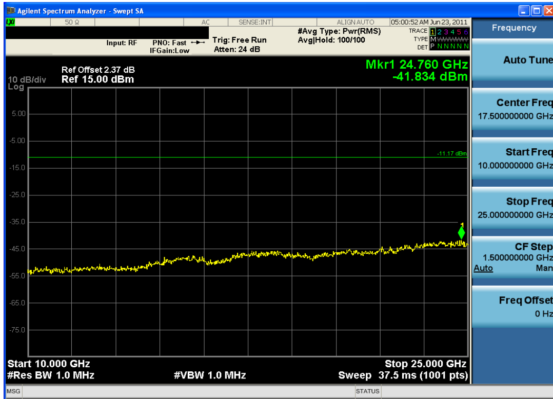
Plot 6-21. Conducted Spurious Plot (Bluetooth, 2Mbps – Ch. 39)
