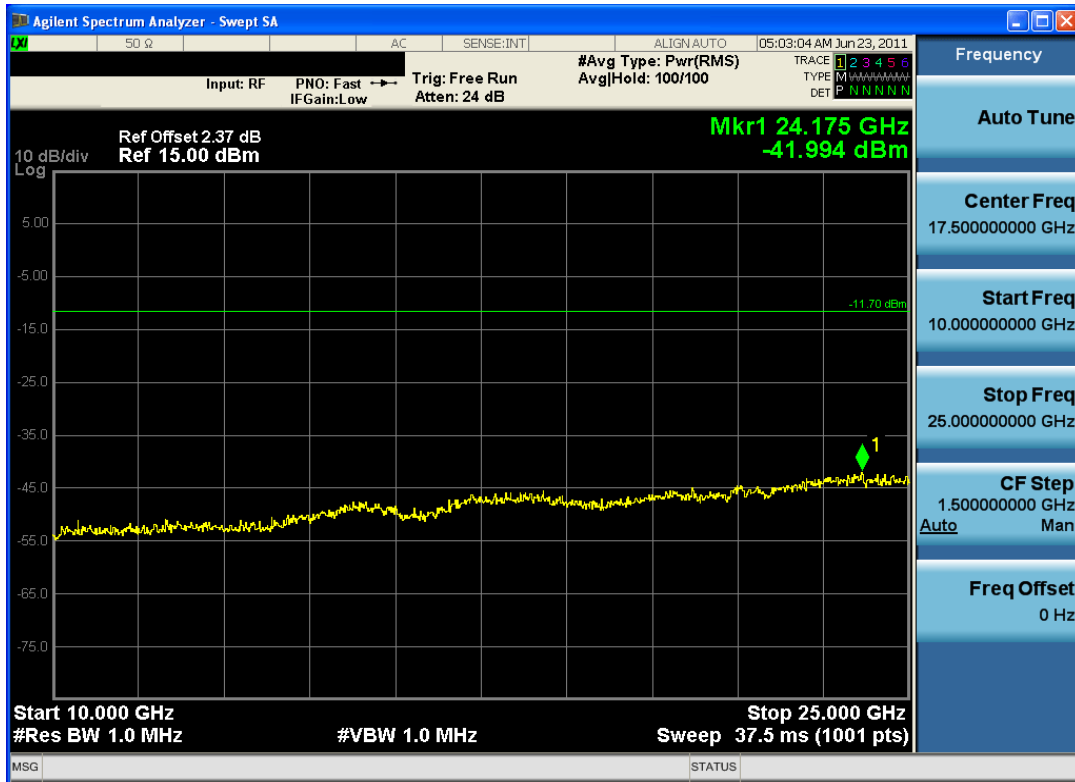
Plot 6-23. Conducted Spurious Plot (Bluetooth, 2Mbps – Ch. 78)
