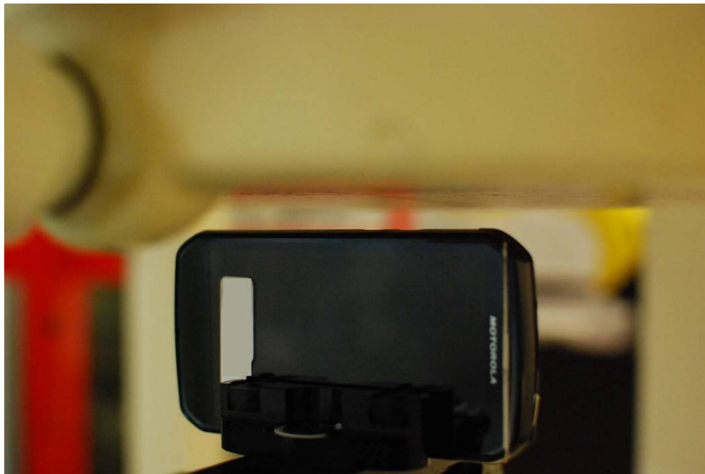
Figure 22-8 SAR Test Setup Photo – Left at 1.0 cm
