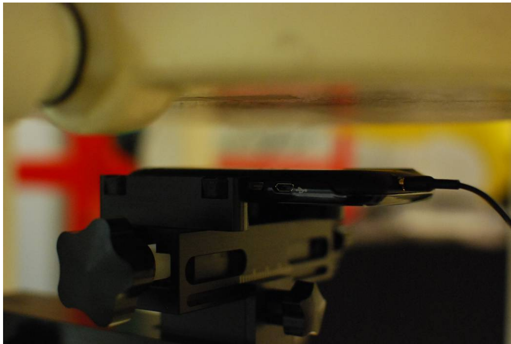
Figure 22-10 SAR Test Setup Photo – Body-Worn at 2.5 cm
