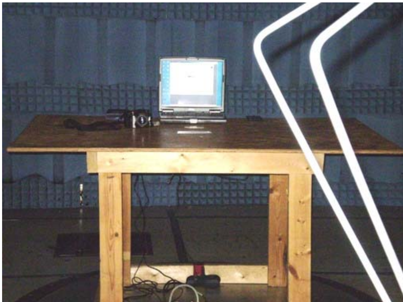
Figure 2: Part 15B, Computer Peripheral Test Set-up.
