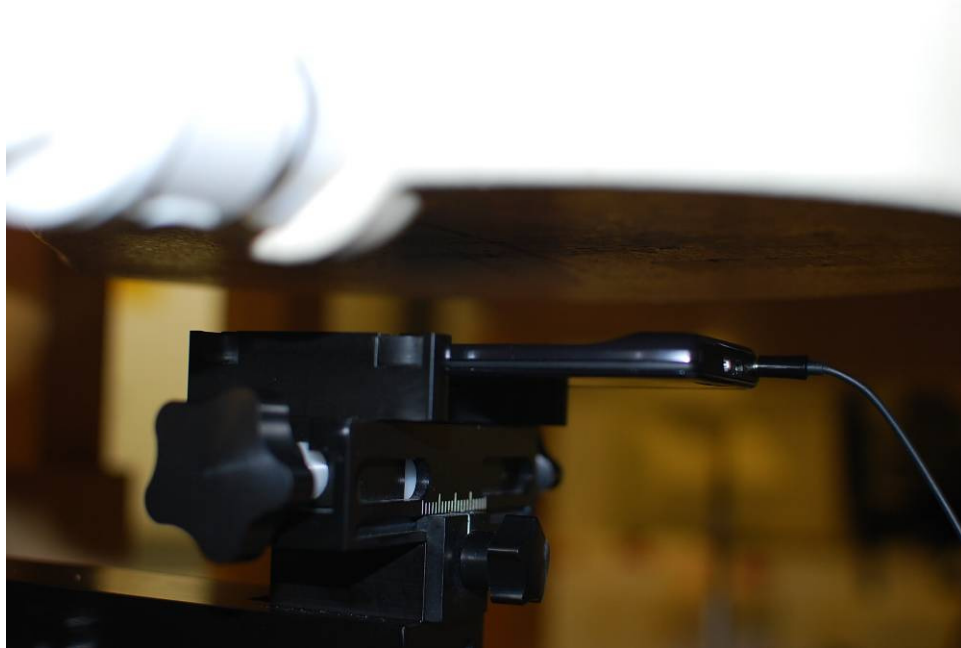
SAR Test Setup Photo 5- Body-Worn Back at 2.5 cm
