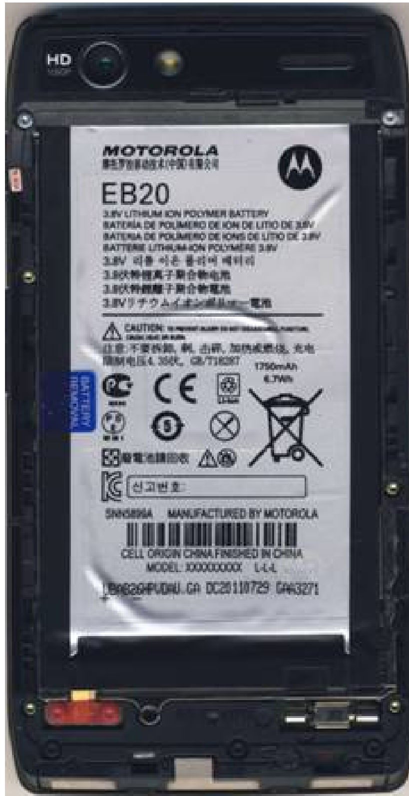
Photograph 9-4: Housing Interior, Showing Battery and Antennas (at the periphery).
