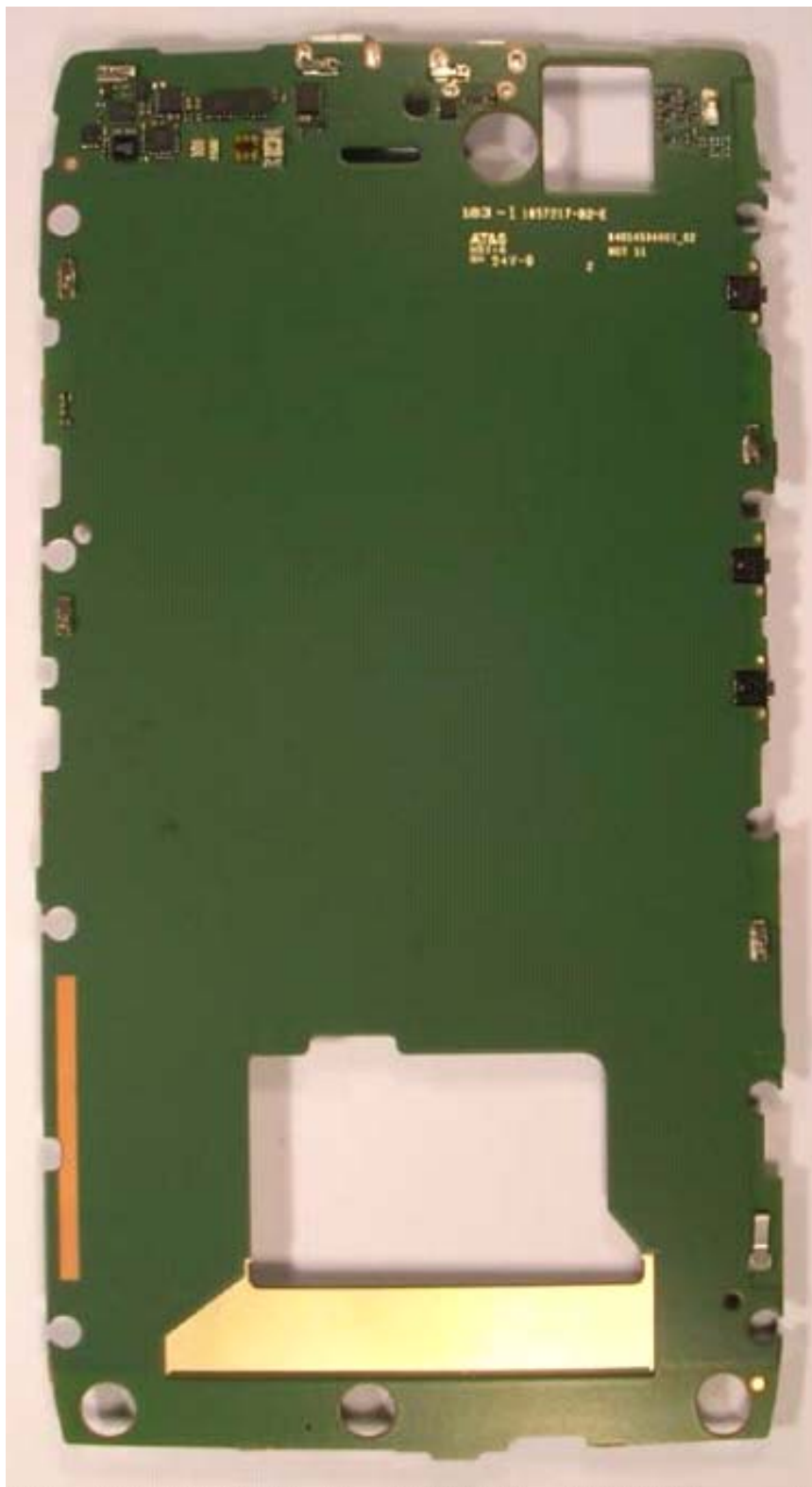
Photograph 9-3: Back side view of the device's PC Board, No Shielding in Design.
