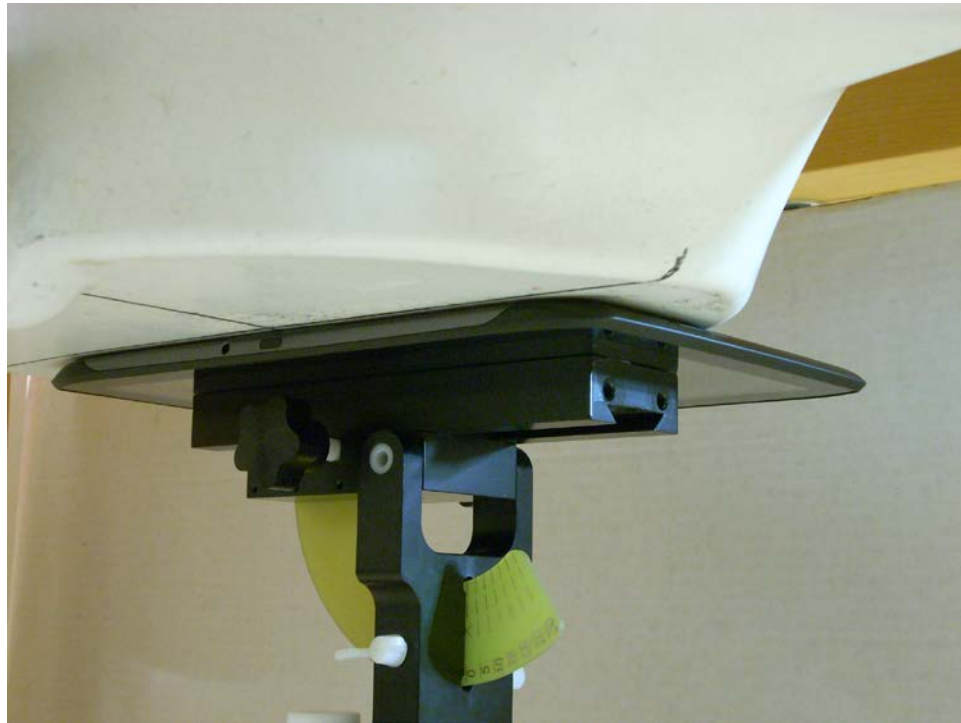
SAR Test Setup Photo 1 - Back at 0.0 cm
