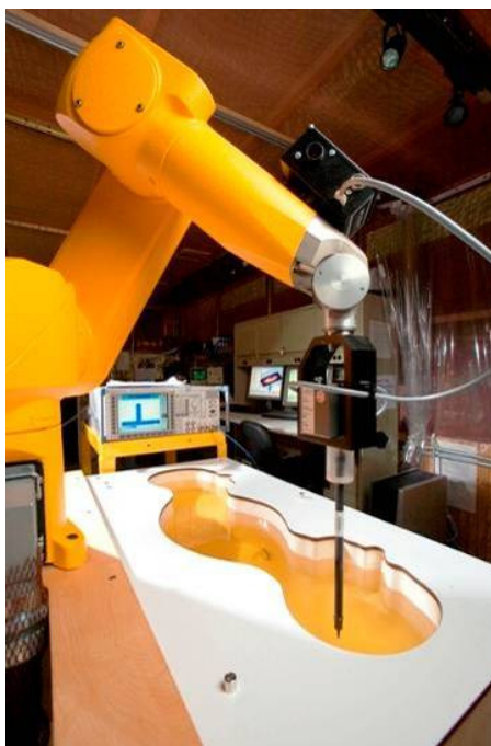
Figure 4-2 SAR Measurement System
