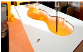
Figure 6-2 SAM Phantom with Simulating Tissue
