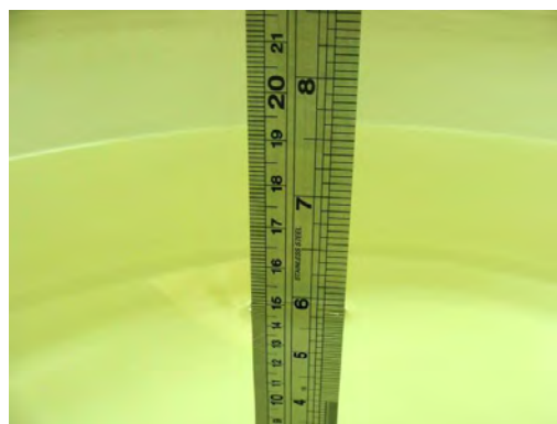
Fig 6.2 Photo of Liquid Height for Body SAR
