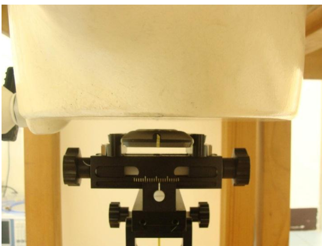
Back of the DUT with Phantom 1 cm Gap (DUT without Earphone)
