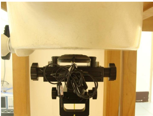
Back of the DUT with Phantom 1 cm Gap (DUT with Earphone)
