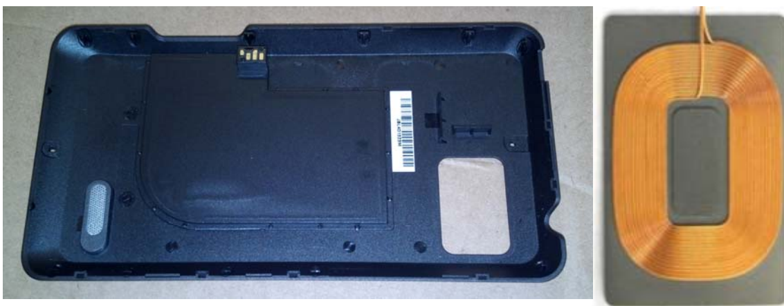
INDUCTIVE BATTERY CHARGING DOOR, AND EMBEDDED PICK-UP COIL
