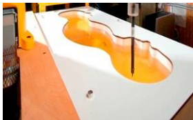
Figure 6-2 SAM Phantom with Simulating Tissue
