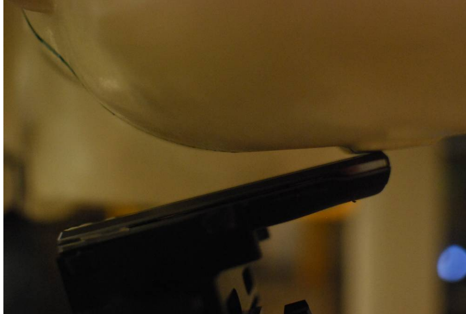
SAR Test Setup Photo 5 – Left Tilt with Inductive Cover
