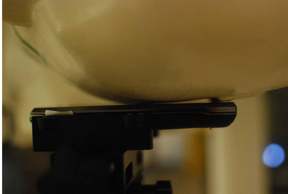
SAR Test Setup Photo 3 – Left Touch
