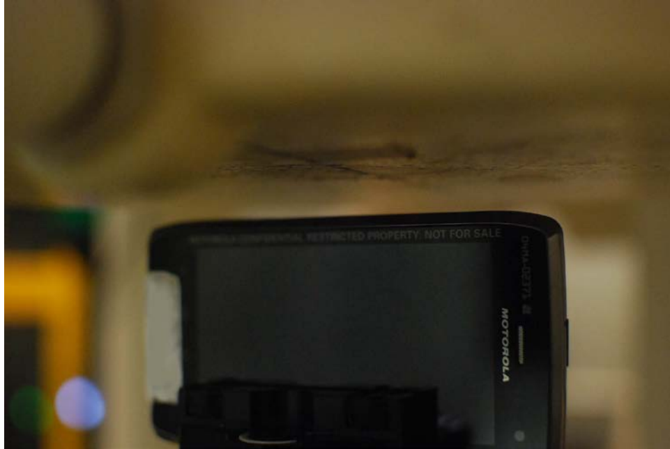
SAR Test Setup Photo 11 – Left at 1.0 cm
