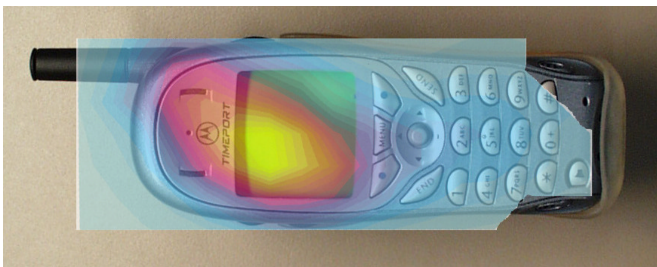
Figure 7. 1900MHz Contour Plot Overlaid on Face of Phone.
